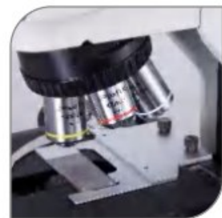
High numerical aperture semi-Apochromat objectives
