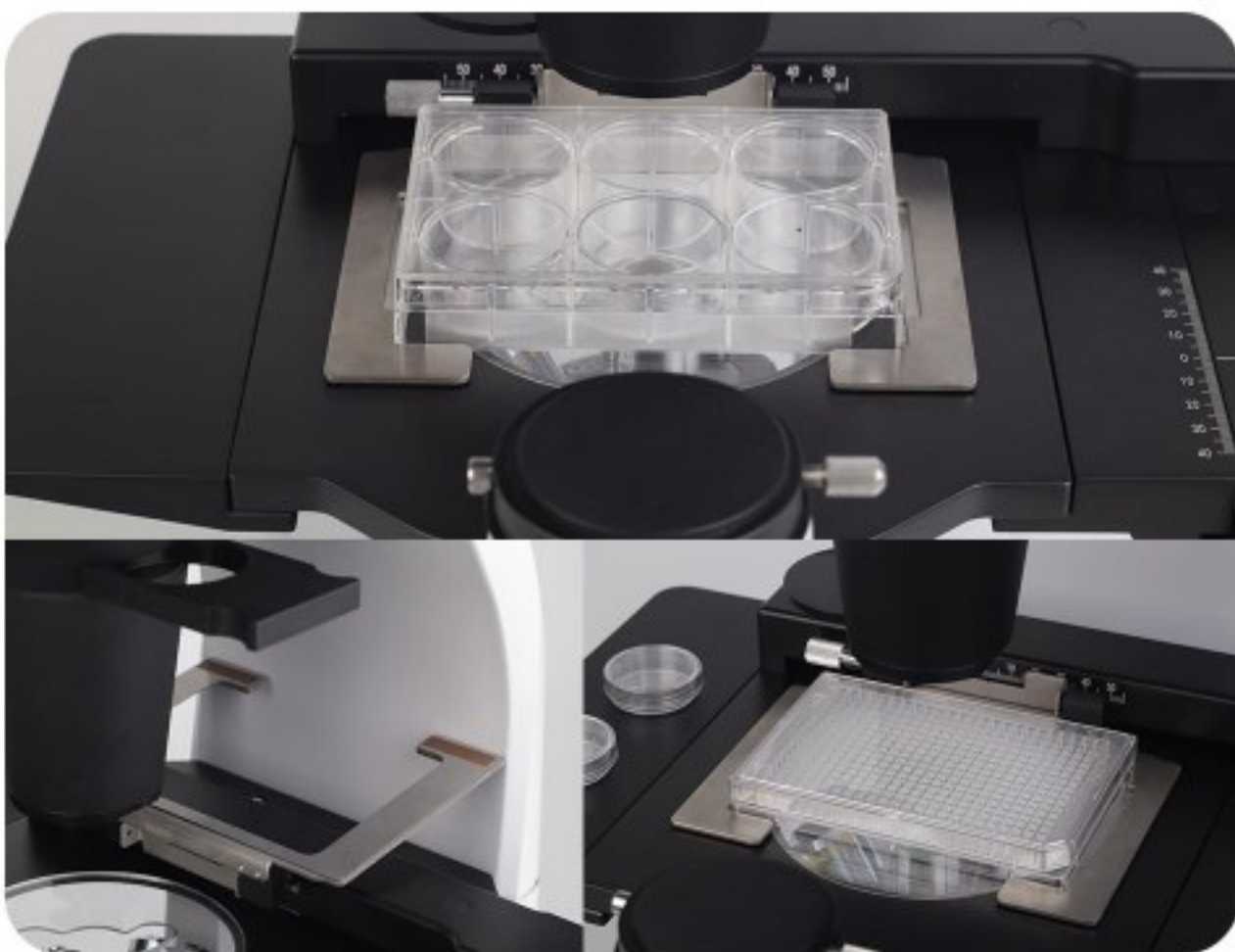
Expandable stage, reversible sample holder
